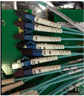
3 = IpGBT11 (COLUTA16) uplink 4 = IpGBT16 (COLUTA20) uplink 5 = IpGBT14 (COLUTA17) uplink 12A = IpGBT13 uplink 6A = IpGBT13 downlink 12B = IpGBT12 uplink 6B = IpGBT12 downlink
