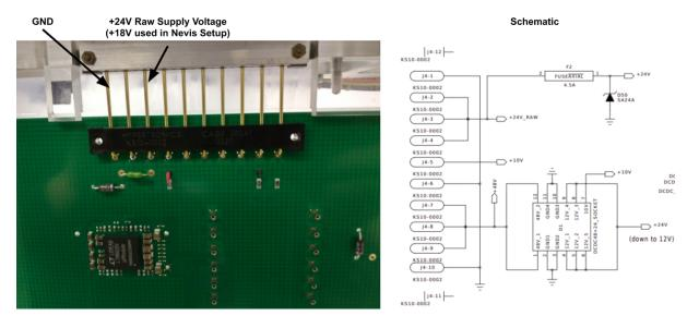
For reference the voltage supply connection to the slice testboard as used in the Nevis test setup is shown here.
